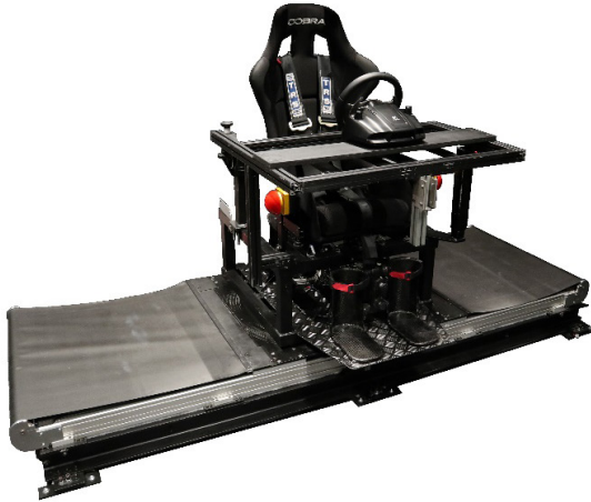
Figure 1.9. Linear motion platform used for closed-loop steering experiments. During the experiment, participants are seated with their interaural axis aligned with the motion axis of the platform, such that they are laterally translated, and rotate a steering wheel to control the sled velocity. Experiments are done in darkness, and participants wear headphones to mask any auditory cues.
