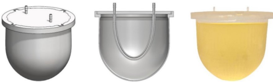
Figure 6.2: Design and setup of the breast perfusion phantom. The schematic illustrations (left and center) show the phantom's structure and position of components, while the right image displays the actual phantom filled with olive oil to mimic fatty tissue.
