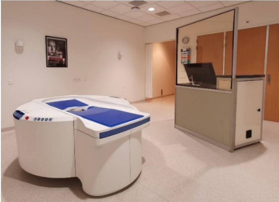
Figure 4.1: Dedicated bCT system installed at Radboudumc and used for this work. The system has a length of 205 cm with a maximum width of 160 cm. The operating console, located to the right in Figure 4.1, comprises a standard computer and monitor with a user interface for image acquisition and reconstruction.
