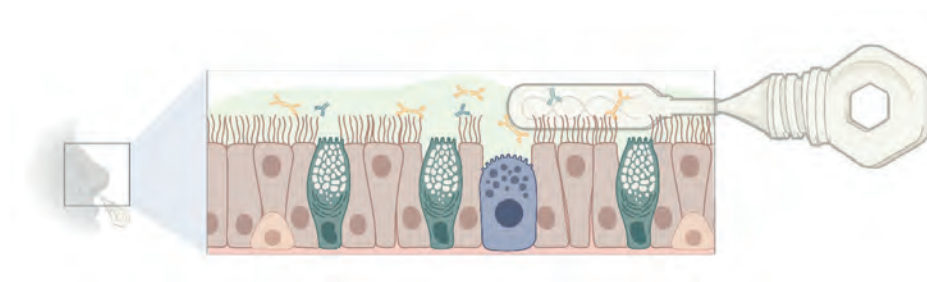
Figure 3: Mucosal lining fluid sampling. A nasosorption strip is inserted into the nose for 60 seconds. It will absorb the mucosal lining fluid, enabling the assessment of nasal antibodies. Created in BioRender. Fröberg, J. (2025) https://BioRender.com/n46o313
