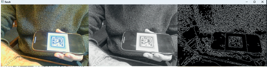
Figure 3. Processing stages: (a) raw image, (b) grayscale conversion, (c) Canny edge output.
