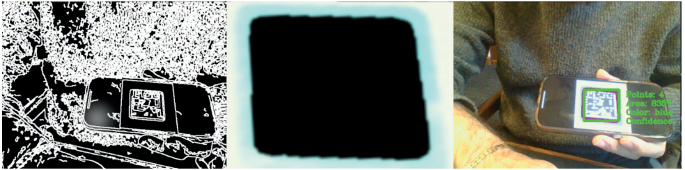
Figure 4. Example of contour selection and bounding-box detection on a colored tag.
