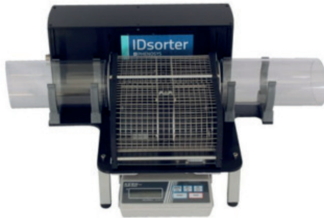
Figure 3. IDsorter automated sorting system developed by Winter and Schaefers. Designed for identifying and separating individually tagged rodents in laboratory settings.
