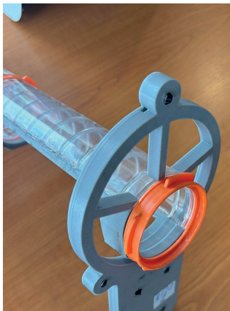
Figure 4. RFID antenna mounted horizontally and pressure-fitted over the FPI tube for optimal signal detection at tube entry.
