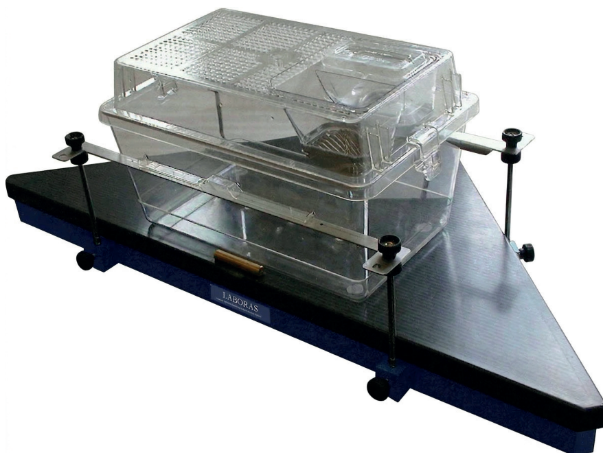
Figure 2. LABORAS system for automated behavioral recording. Image shows the vibration-sensitive platform with home cage setup designed to detect and classify rodent behaviors automatically. Source: Metris B.V., Netherlands.
