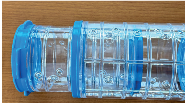
Figure 2. Binocular FPI connector tube, designed for secure and transparent passage between cages in the automated system.
