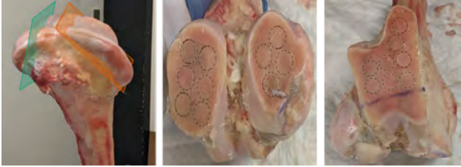
Figure 2-1: Overview of coring and cutting locations. On the left picture, the cutting planes on the distal femur are shown. The green plane shows the cut through the cortex of the condyles and the orange plane shows the trochlear cut. In the middle image, the drilling holes and thereby specimen locations in the condyles. On the right, the specimens locations in the trochlea of this particular bovine femur are displayed.
