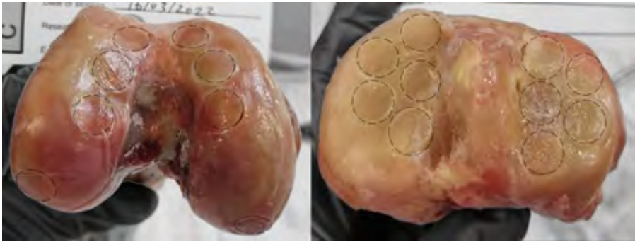
Figure 3-2: Anatomical locations of cylindrical trabecular bone specimens harvested from the distal femur (left) and proximal tibia plateau (right). Dashed circles indicate the coring sites, distributed across anterior, posterior, medial, and lateral regions to ensure representative sampling of load-bearing areas.
