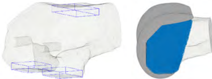
Figure 4-3: Left: The three regions of interest (anterior flange, medial posterior condyle, and lateral posterior condyle) to determine the average BMD and equivalent von Mises stress. The ROI was defined from the bone-implant interface to a depth of 5 mm in the femur. Right: The region of the bone, highlighted in blue, over which the strain energy is determined, is situated between the anterior and posterior surfaces of the implant.
