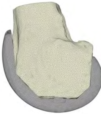
Figure 1-4: Finite element model of a femur with a femoral component, used to study primary fixation. The smaller elements on both the bone and the implant represent the mesh used for detailed analysis of micromotions and implant-bone interaction during the early fixation phase.
