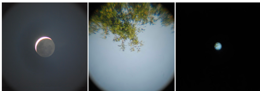
Figure 2: The two-day-old Moon (left) and a terrestrial scene (centre) observed through a Keplerian telescope with a 50 mm diameter objective lens and a magnification of 20 times. The objective and ocular lenses have focal lengths of +1000 mm and +50 mm, respectively. Right: the terrestrial scene observed with the same objective lens, but using a concave ocular lens (that is, the Dutch/Galilean configuration) with a focal length of -50 mm, also magnifying 20 times. The latter would not show the entire Moon, even at this modest magnification. Photos by the author.
