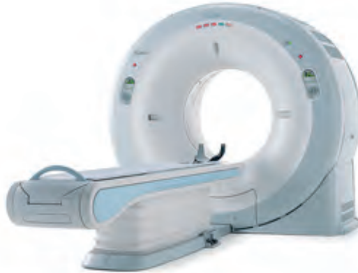
Figure 1.2: Computed tomography scanner. An X-ray tube and an oppositely placed detector are situated within the circular gantry at the head of the scanner bench. The detector measures the X-ray beam attenuation of a subject on the bench creating a projection image. The gantry internals can rotate at approximately two to three revolutions per second. Image source: https://us.medical.canon/ (September 2022). Copyright: Canon Medical Systems.
