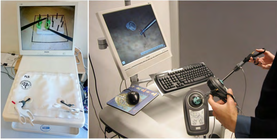
Figure 2. Training stations: The FLS videotrainer and the LapSim virtual reality trainer.
