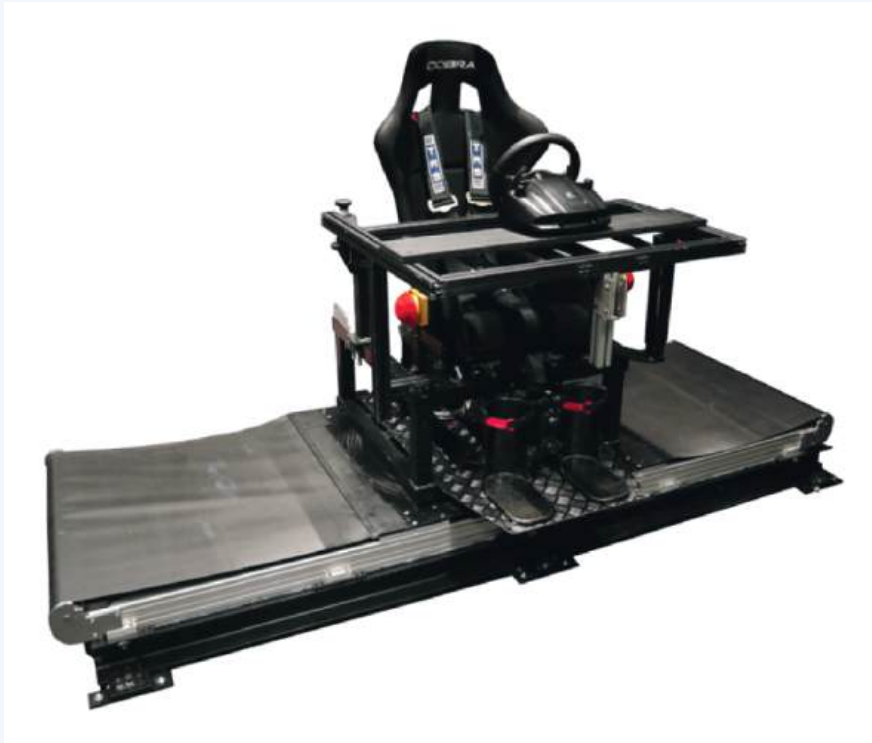
Figure 1.7. The vestibular sled setup, consisting of a chair on top of a linear motion platform. Image reproduced (with permission) from van Helvert (2025).
