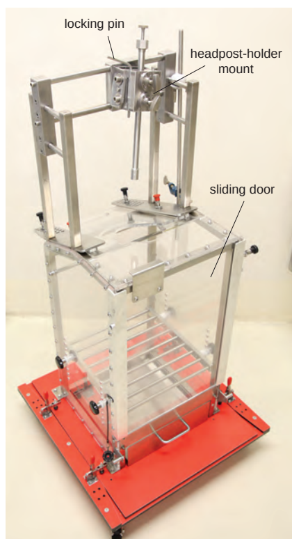
Suppl. Figure 2.3. Primate chair and headpost-holder mount. Photos of the primate chair and the headpost-holder mount. The headpost holder is secured to a mount that is attached to the primate chair. The orientation of the mount can be adjusted to accommodate oblique headpost-holder orientations.
